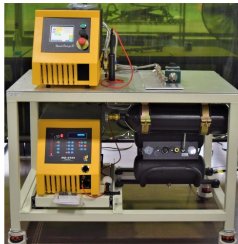
Leak ID Station with Single Table
