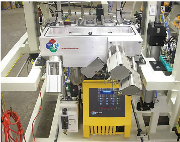
This leak test system for fuel rails includes a hard-vacuum test chamber, vacuum pump and helium mass spectrometer. Photo courtesy Vacuum Instrument Corp.
