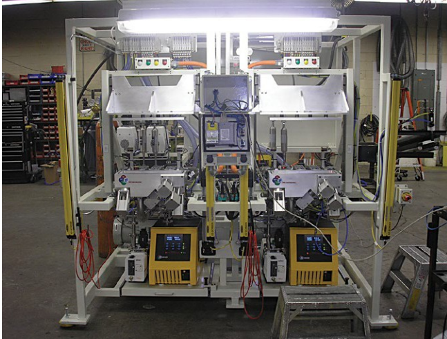
High-pressure, direct-injection fuel rails have a leak rate spec of 10^{-4} atmospheric cubic centimeters per second. Photo courtesy Vacuum Instrument Corp.
