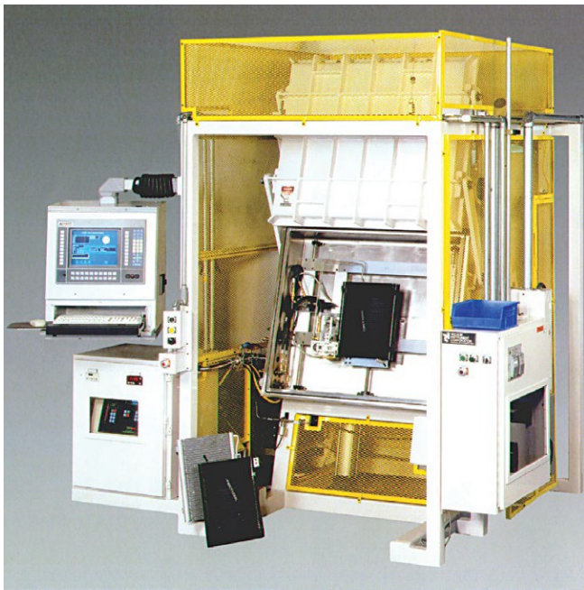
An air-conditioner condenser is in position to be leak-tested in a helium hard-vacuum system. Photo courtesy Vacuum Instrument Corp.
