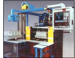
Fuel Tank Assembly Test
